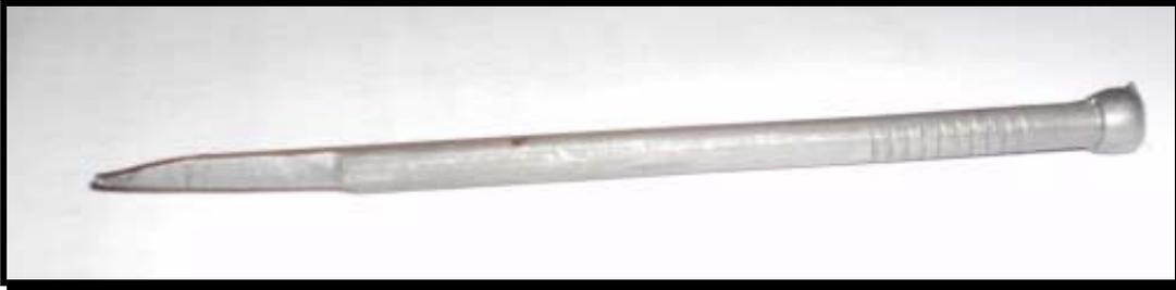
3. Remove the blade pin attached to the orange/blue wire in the connector at the main harness end of the sub-harness. Only remove the blade pin attached to the orange wire with the blue tracer. This is the signal wire from the NC30 speed restrictor. You will need the above tool to depress the locking tab to permit removal of the blade pin from the connector (see picture). It is a finicky job so be careful and do not damage the blade pin. It should look like this now.
