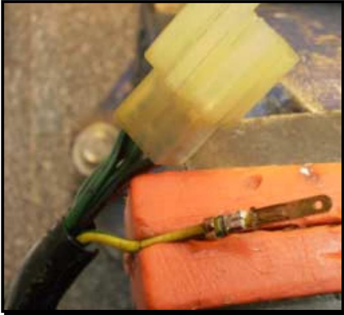
7. Check the locking tab on the blade pin and make sure it is sticking out a couple millimetres.
